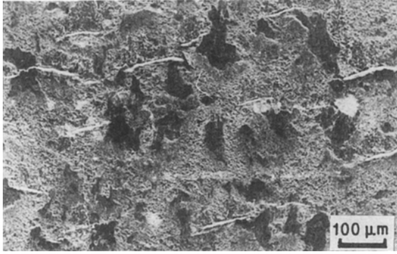
Figure 12 SEM micrographs showing microcracks and associated interlocked areas in an SPL shear failed specimen.
